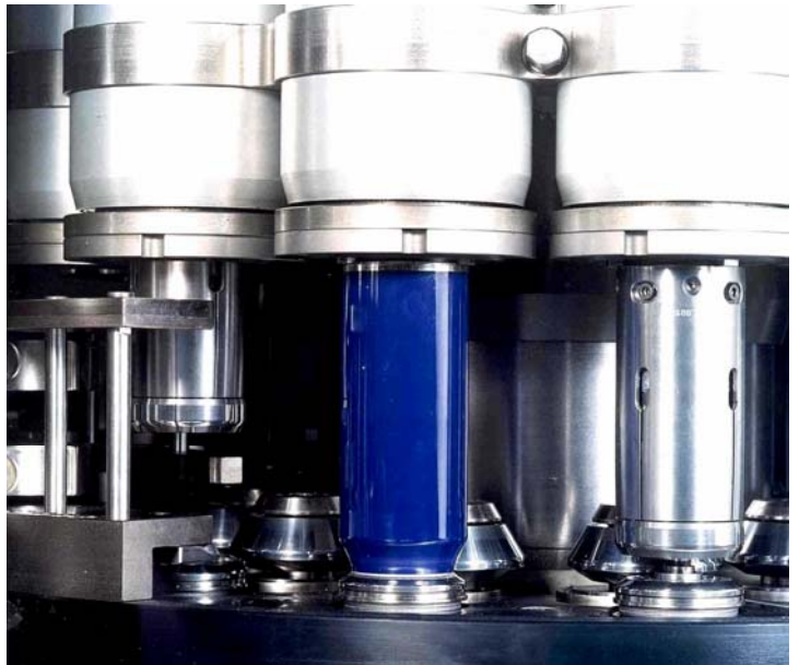
Spin-flow necking process
